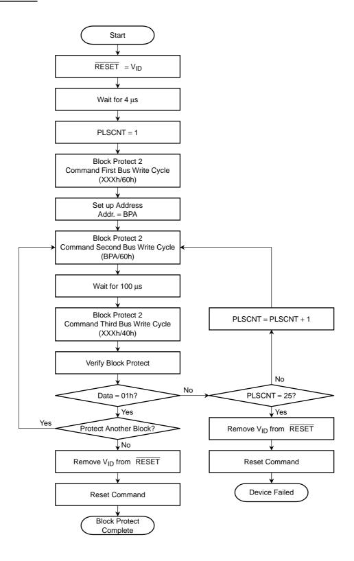
BPA: Block Address and ID Read Address (A6, A1, A0) ID Read Address = (0, 1, 0)
