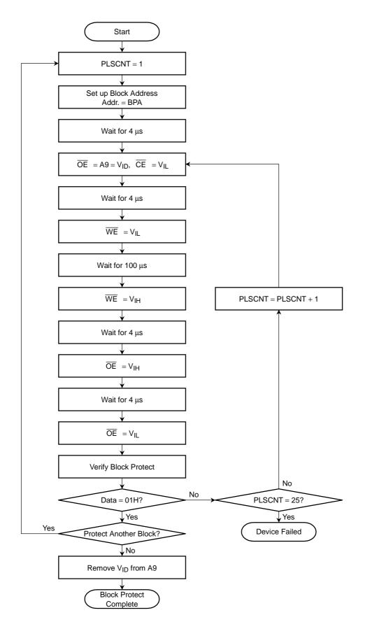
BPA: Block Address and ID Read Address (A6, A1, A0) ID Read Address = (0, 1, 0)
